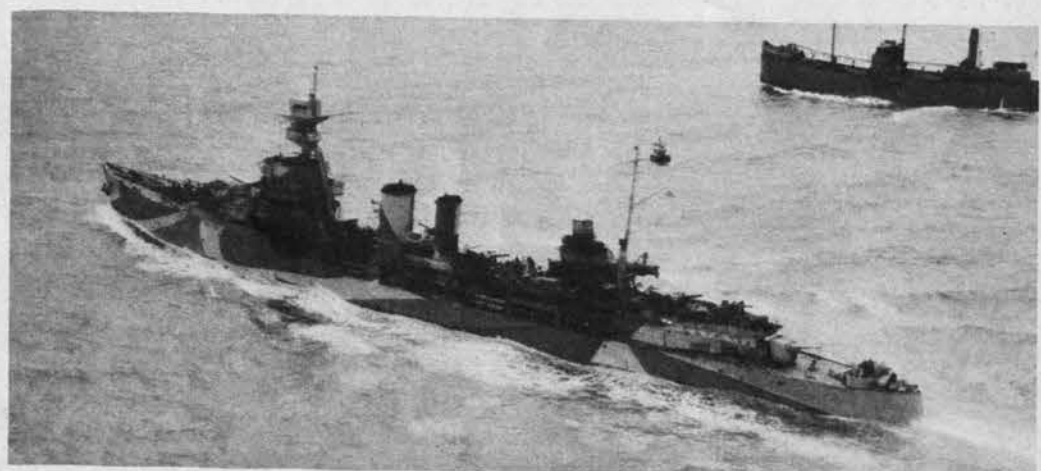
Light superstructure, closely spaced stacks of unequal width, and single shield gun mounts are typical of the four British World War I cruiser classes—Dragon, Caledon, Ceres and Carlisle.
